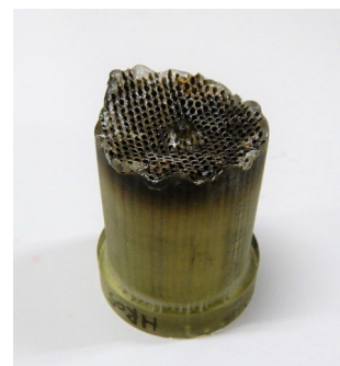
Fig. 28. The side of the fuel after the visualization experiment ( Test 2 )
