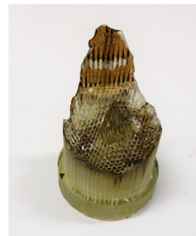
Fig. 27. The side of the fuel after the visualization experiment ( Test 1 )
