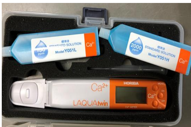
Figure 4. 4: Calcium ion meter with standard solutions for calibration.
