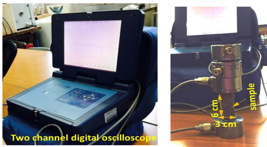
Figure 5. 7: Ultrasonic measurement of fiber treated MICP specimen.
