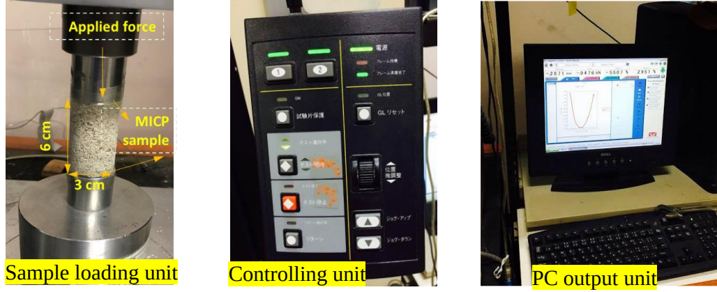
Figure 5. 6: UCS machine (Instron-2511-308 load cell).
