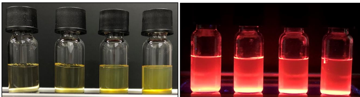
Figure 2.6. Aqueous SiQD solutions under a) white light and b) UV light
