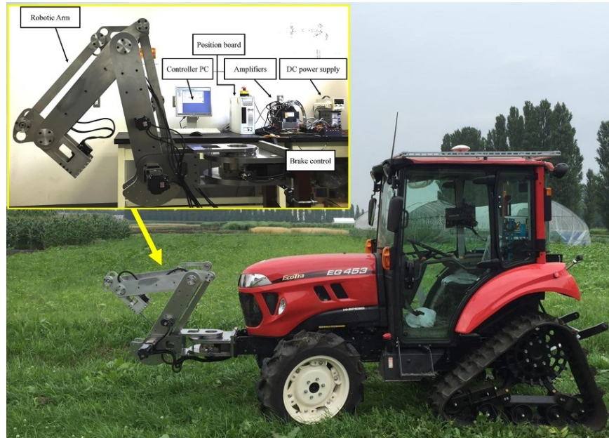
Figure 14. Designed robotic arm (RAVeBots-1)
