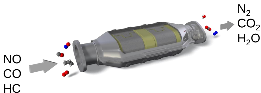
Scheme 1. Three-way catalytic convertor
