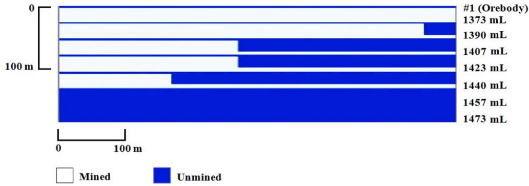
Fig. 4.1 Input model for the numerical analysis (the mine layout as of July 2016).
