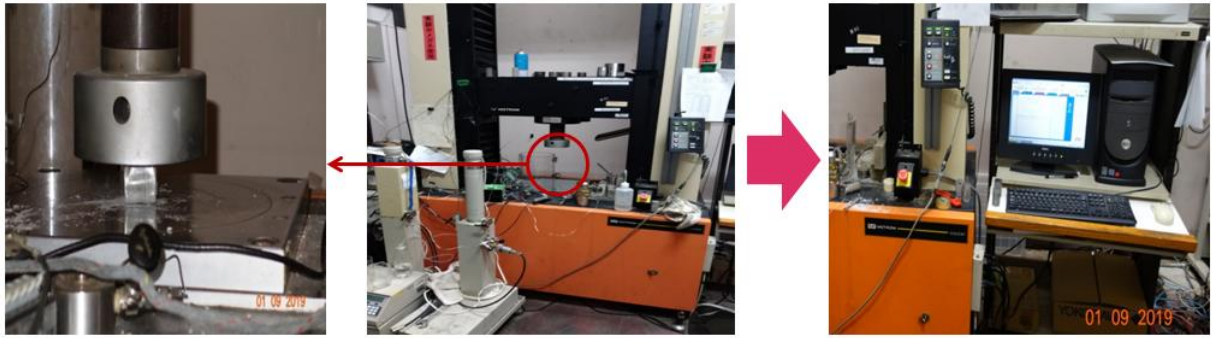
Fig 3.2 Instron loading frame used in the experiment.
