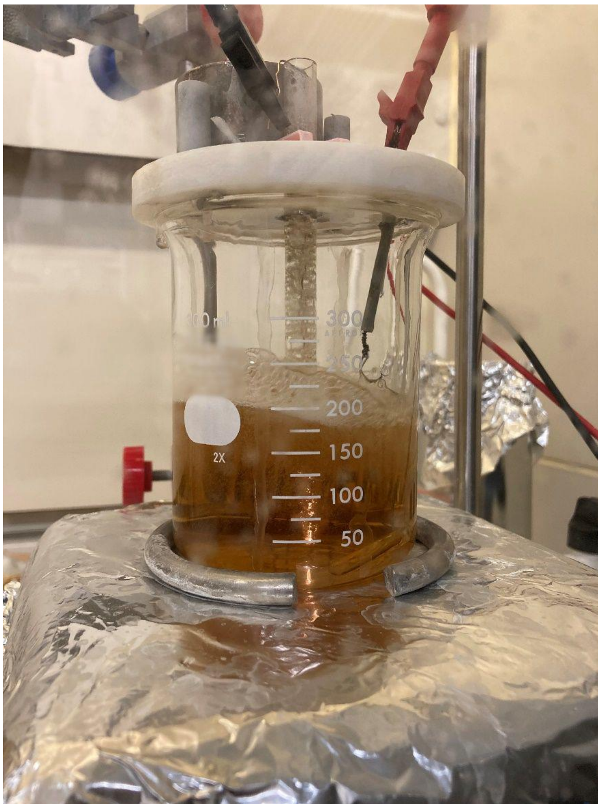
Figure 2.7. Image of dark yellow supernatant of SPP synthesis of b-TiO 2 in water-ethanol electrolyte.
