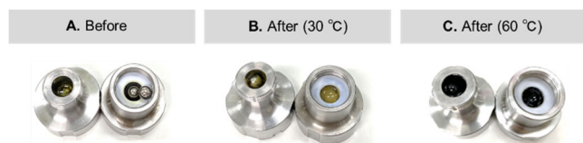
Figure 2. Reaction mixture (A) before ball milling, (B) after ball milling at 30 °C (entry 3, Table 1), and (C) after ball milling at 60 °C (entry 4, Table 1).
