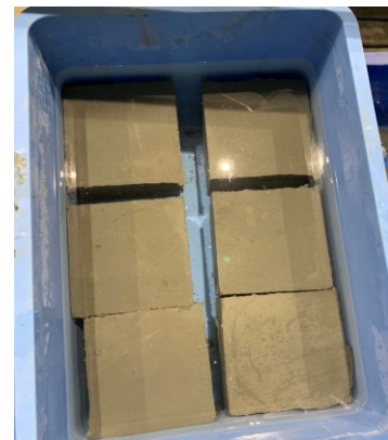
(e) Curing in wet condition
