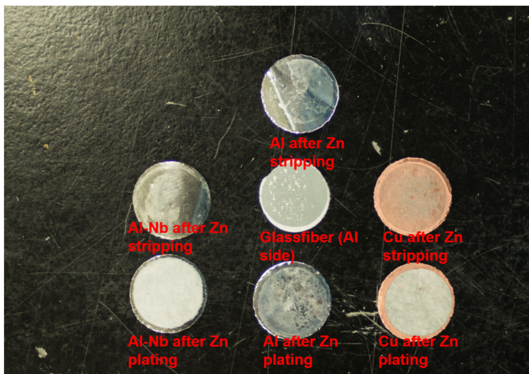
Figure S9. Optical photos of different metal substrates after Zn plating or Zn stripping.
