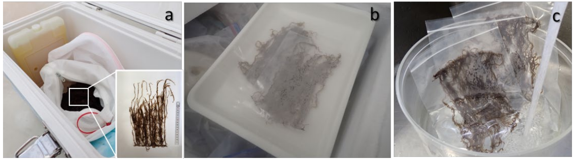
1 2 Fig. S1 The process of freezing and thawing a net piece sample. (a) Transported a net 3 piece sample into the laboratory in the refrigerated condition with ice packs, (b) Sealed 4 in a zipper bag and frozen at -30^{\circ}\text{C} , (c) Thawed under running water.
