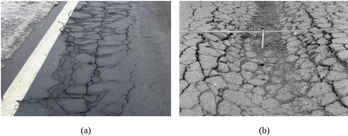
Figure 1-1 Types of pavement damage in in seasonally cold region ((a)Fatigue cracks; (b) Rutting).
