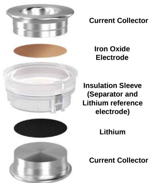
Figure 6.2 Schematic of lithium ion battery half-cell.
