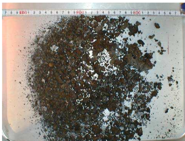
Figure 4.8 Photograph of appearance of desulfurization slag after treatment (condition A)
