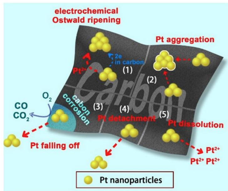
Figure 1-6. Schematic diagram of the performance loss mechanism of Pt/C catalysts in ORR.
