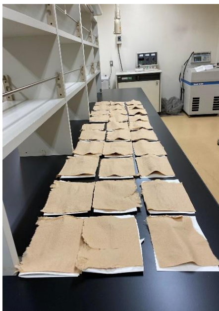
Fig. 3.2 Soil sample air-dried at Toyoda laboratory.
