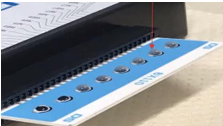
Figure 4.2 The 8-channel screen-printed carbon electrode (SPCE) system with carbon as working and counter electrode, and Ag/AgCl as reference electrodes.
