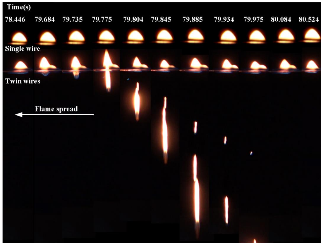
(a) Single-wire and twin-wire conditions at \theta=0^\circ
