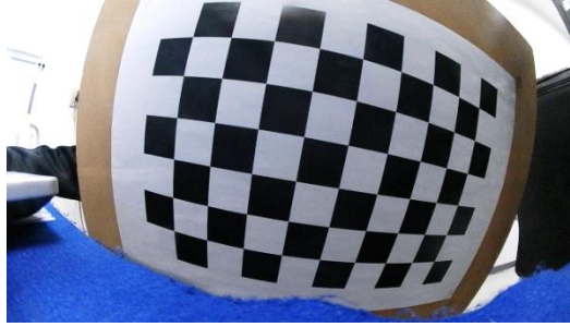
Figure 3.3. 9x6 grid chessboard used to find the camera intrinsic parameters
