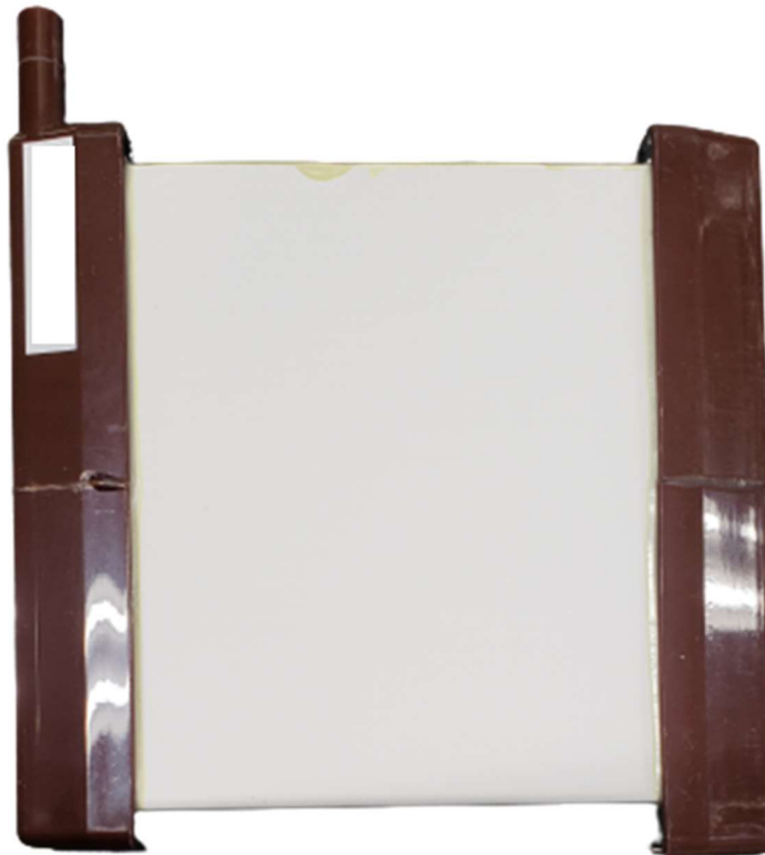
Figure 2.4-1: Flat-sheet ceramic membrane used in the experiments.
