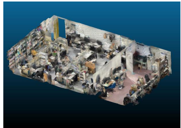
Fig. 4 Indoor image data (colored point cloud) of acquired using Scaniverse
