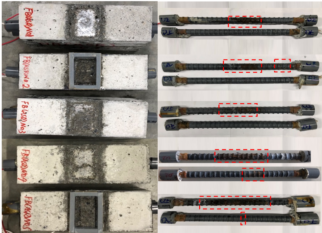
(d) Appearances of FBA concrete (FBA1, FBA2, and FBA3 1031 days; FBA4 and FBA5 on 692 days), rebars on the split date
