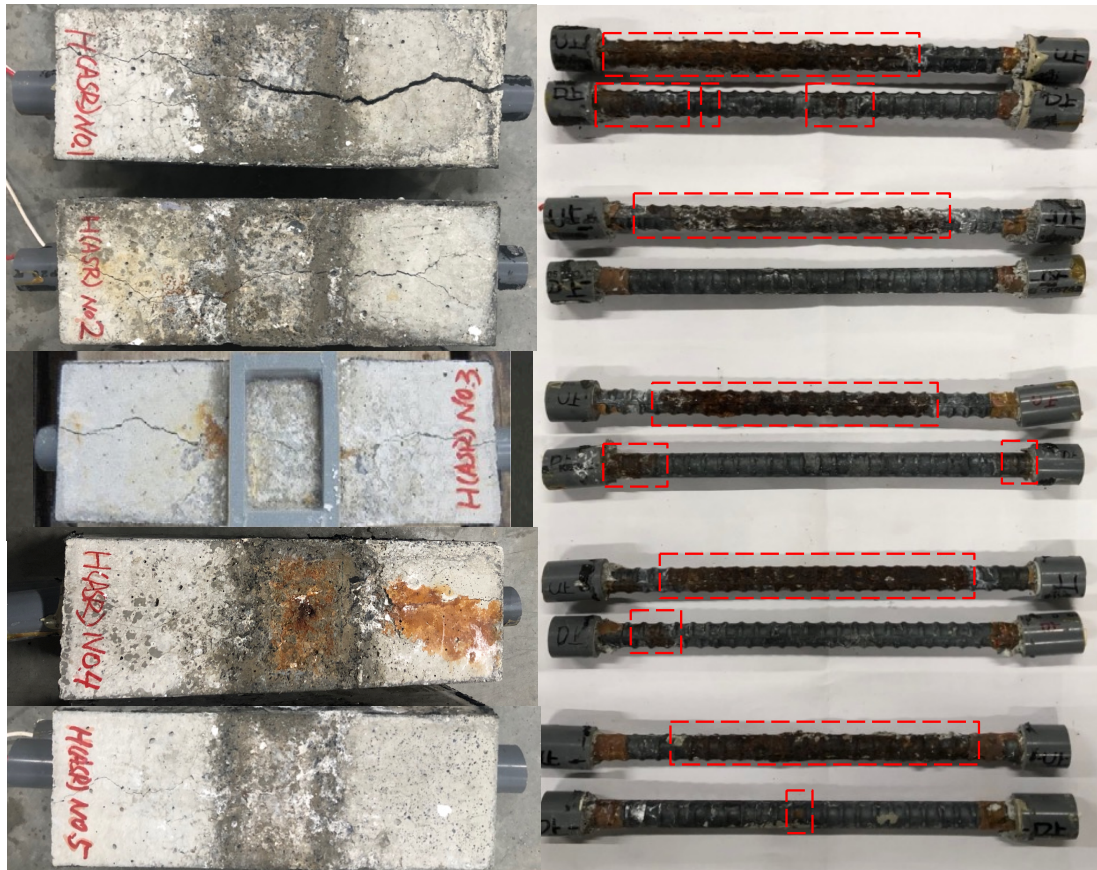
(b) Appearances of HA concrete (HA1, HA2, and HA5 on 1083 days; HA3 on 490 days and HA4 on 663 days), rebars on the split date
