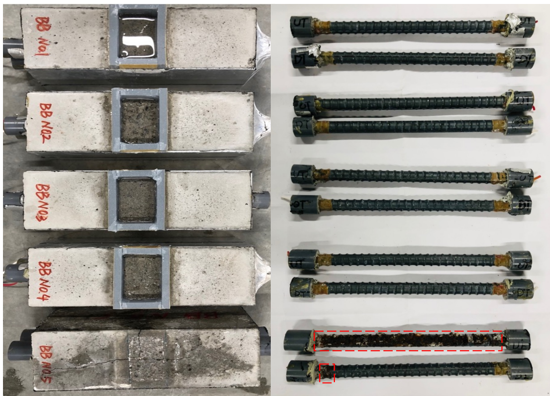
(e) Appearances of BB concrete at 1065 days (BB5: 678 days), rebars on the split date
