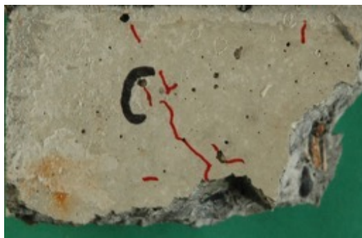
(c) ASR cracks on the "A" part
