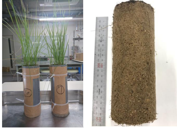
Fig. 10 Example of grassed soil specimen.
