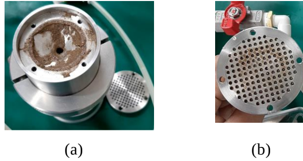
Fig. 5.1. Fines trapped in (a) pedestal, and (b) porous plate.
