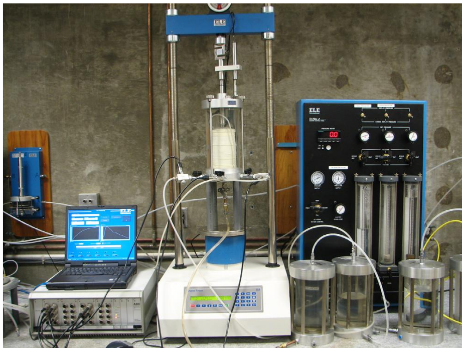
Fig 2.4. Suffusion experimental set up used by Xiao and Shwiyhat (2012).
