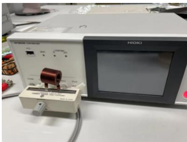
Fig. 4-18. Photograph of LCR meter and inductor
