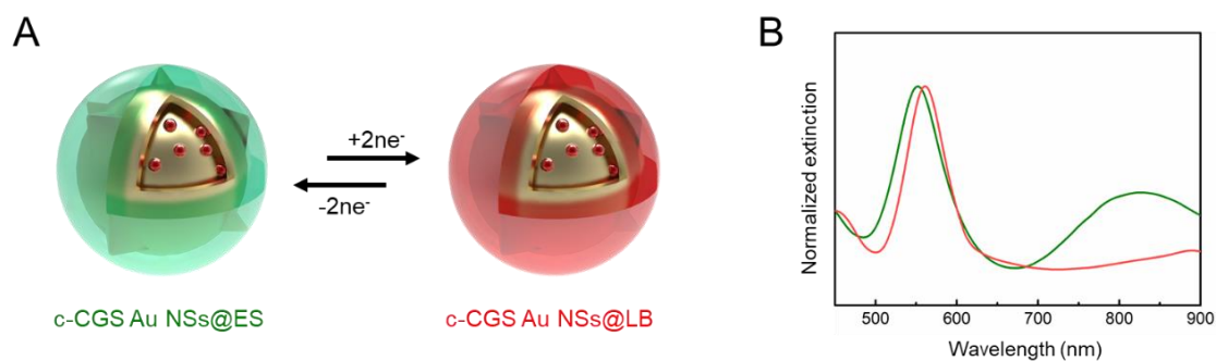
Figure 3.14 (A) Schematic illustrations and (B) normalized extinction spectra of the conversion between c-CGS Au NSs@PANI (ES) and c-CGS Au NSs@PANI (LB) .
