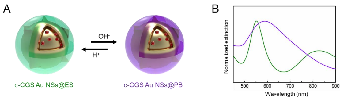
Figure 3.6 (A) Schematic illustrations and (B) normalized extinction spectra of the conversion between c-CGS Au NSs@PANI (ES) and c-CGS Au NSs@PANI (PB) . (C) Schematic illustrations and (D) normalized extinction spectra of the conversion between c-CGS Au NSs@PANI (ES) and c-CGS Au NSs@PANI (PB) .
