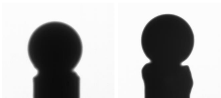
Fig. 4-4 Comparison of rigid sphere images using backlight method (right figure) and shadowgraph method without filter (left figure).
