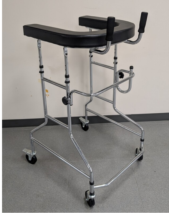
Figure 1.1: Forearm support walker with adjustable height support platform and four-wheel base.
