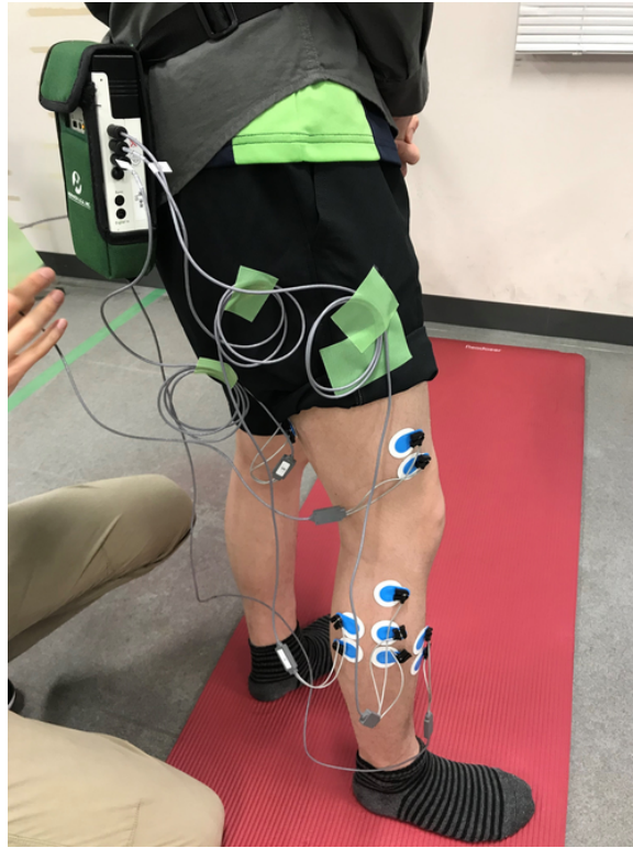
Figure 4.2: Appearance of myoelectric measurement.
