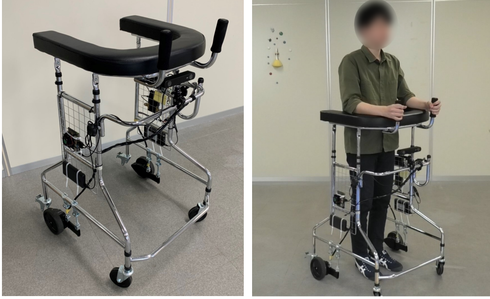
(a) Metal walker utilized in the experiment. (b) Condition in which the body weight is supported.
