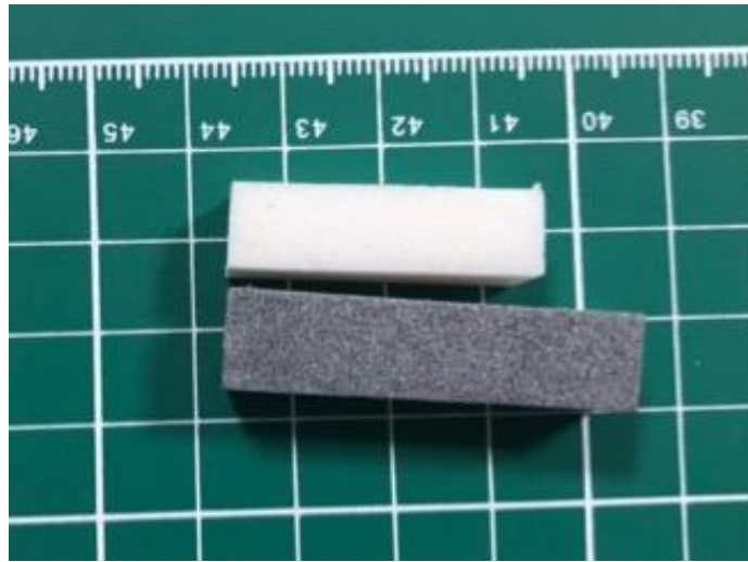
Figure 28. Samples – above the white one: extruded polystyrene foam (XPS), bottom the black one: extruded polystyrene foam with graphite
