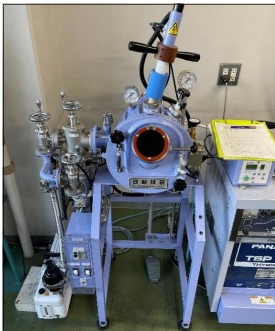
Fig 2.1 Arc melting furnace with an enclosed crucible.
