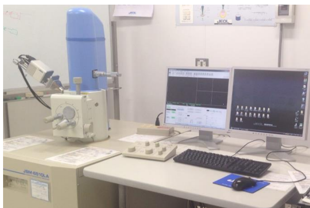
Fig 2.4 The figure of scanning electron microscopy (SEM).
