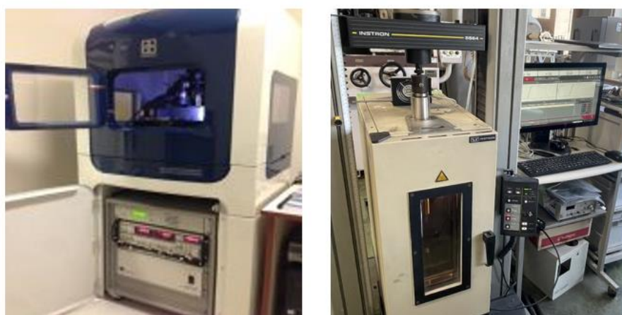
Fig 2.9 Nanoindentation test machine(left) and tensile test machine(right).
