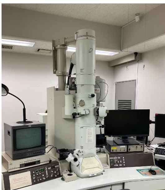
Fig 2.6 The figure of TEM(JEOL JEM-2010).
