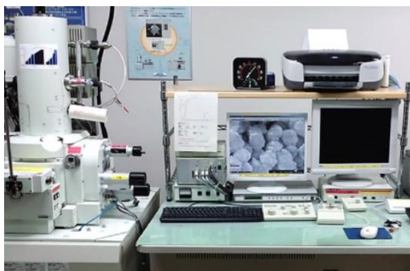
Fig 2.5 The figure of Electron Backscatter Diffraction (EBSD) facility.
