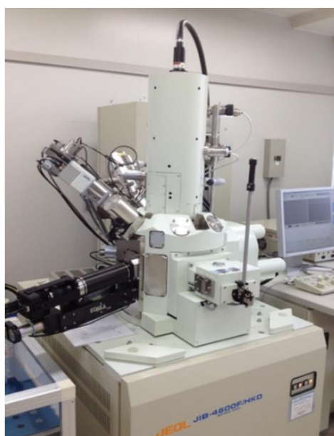
Fig 2.7 The figure of FIB (JEOL, JIB-4601F) facility.
