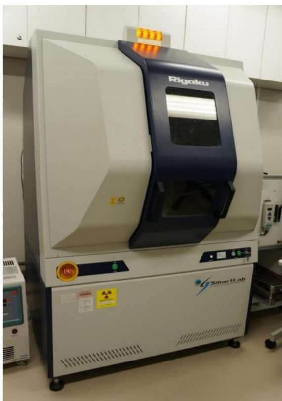
Fig 2.3 The figure of SmartLab XRD.
