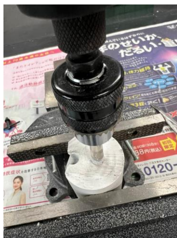
Figure 5.2: Sample extraction using core drilling
