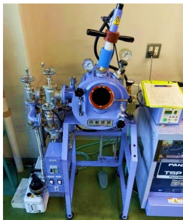
Fig. 2.2 Arc melting furnace with an enclosed crucible.
