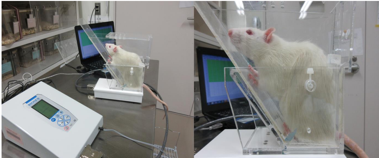
Figure 3. Incapacitance tester for determination of hind paw weight distribution.
