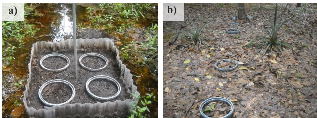
Fig. 2. Experimental scenes of (a) peat decomposition (PD) and (b) total soil respiration (SR).
