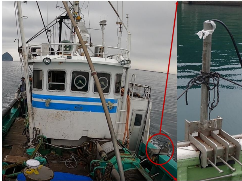
Figure 4-2. Kakutomaru, a purse seine fishing vessel used for the survey, and the installation location of an external quantitative echo sounder.
