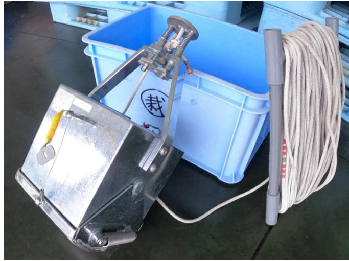
Figure 4-6. An Ekman Barge-type grab sampler manufactured by RIAGO was used to sample the seabed sediments.
