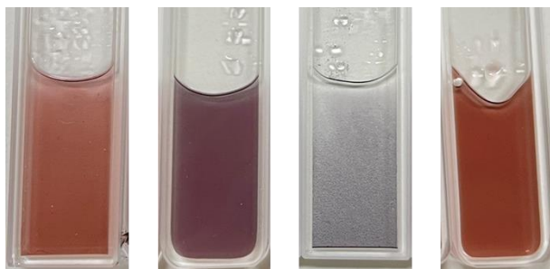
Figure 2-3 The images of AuNRs solution with different DNA concentration. From left to right: no DNA (dispersed), low amount of DNA (assembled), medium amount of DNA (aggregated) and high amount of DNA (dispersed).
