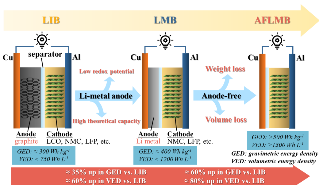
Figure 1-4. The schematic comparisons of LIB, LMB and AFLMB. LCO, NMC and LFP are the abbreviation of \text{LiCoO}_2 , \text{Li}(\text{Ni}_x\text{Co}_y\text{Mn}_{1-x-y})\text{O}_2 and \text{LiFePO}_4 , respectively.
