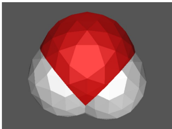
Fig. 2.6 Tesserae of C-PCM (water solvent) cavity for a single water molecule. The red sphere corresponds to the oxygen atom and white spheres correspond to hydrogen atoms. The cavity surfaces consist of small triangles called “tesserae”. The point charges are located at the center of each tessera (not shown in Fig. 2.6). The tesserae data file was created by the Gaussian16 program and visualized by the Geomview program 28 .
