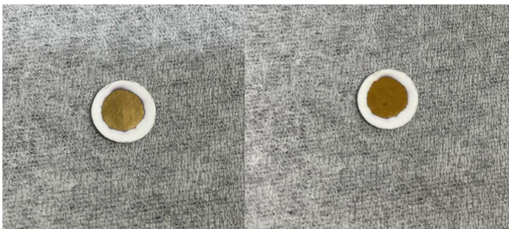
Figure 2.4 Photographs of surface gold coating on a pellet by ion coating (left), followed by further coating with gold paste (right).
