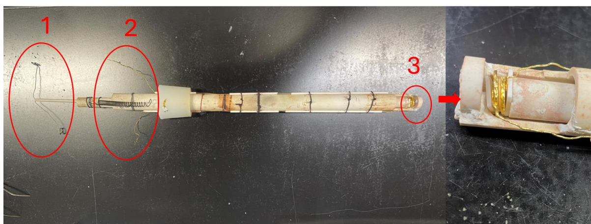
Figure 2.5 Photographs of the setup for electrical conductivity measurements. A pellet is placed between two gold electrodes (3), the cell shell is handmade by alumina. The gold electrodes are connected to the outside through gold wires to facilitate the application of current (2). A simple temperature sensor is placed near the gold electrodes to detect the cell temperature, which is also extended outside with a wire (1). After setting, use a spring to fix to prevent loosening.
