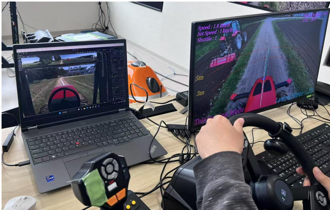
Fig. 5.10. Display image of remote controlling system
