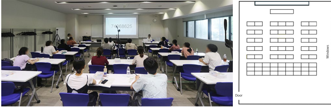
Fig. 3.2. Regular classroom image during the experiment with data loggers (a), regular classroom plan with data logger's positions (b).
