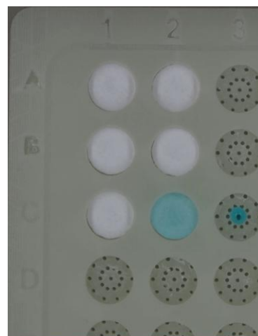
Fig. 3- 6 A 5 \mu L of blue dyes in 10 mM PBS adsorbed well through the paper disc while it did not flow through the microvalves
