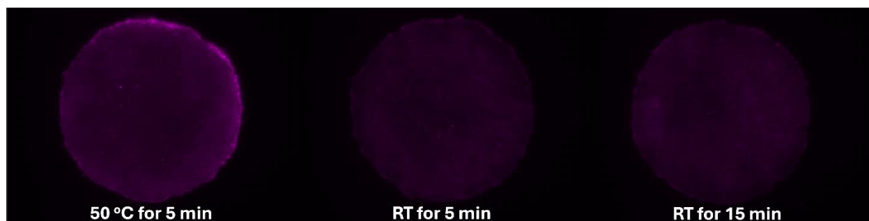
Fig. 2- 3 Fluorescence images for capture antibody immobilized at 50^\circ\text{C} for 5 min, and room temperature at 5 and 15 min. The procedure was done as follow, first 3 \mu\text{L} of 10 \mu\text{g/mL} anti \beta' -c Ab (from rabbit) was added to the detection zone and dried at 50^\circ\text{C} or room temperature. Next the unreacted antibody was washed twice using 15 \mu\text{L} of 0.05% PBST, the paper was blocked using 3 \mu\text{L} of 2% BSA. Then 3 \mu\text{L} of 10 \mu\text{g/mL} Cy5-labeled anti-rabbit antibody was added and incubated 2.5 min at room temperature to attach to the immobilized antibody. Finally, the unreacted cy5 labeled antibody washed twice using 15 \mu\text{L} of 0.05% PBST.
