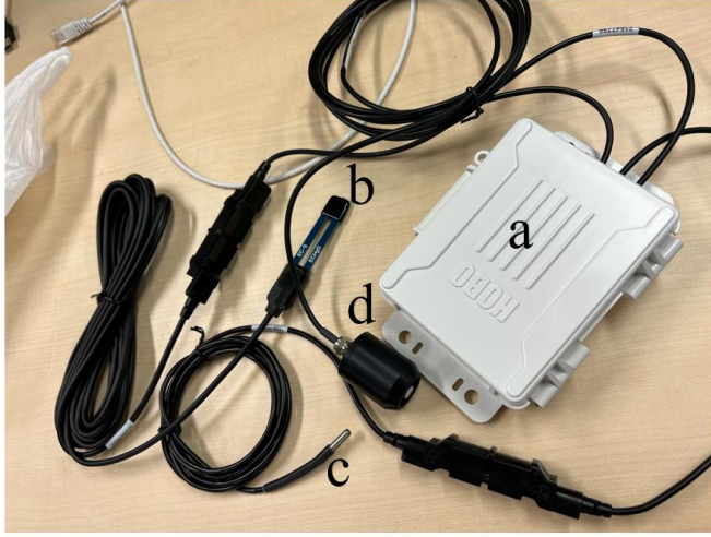
Figure 3.1.4.1: Equipment: (a) Data micro station loggers (HOBO H21-USB), (b) 5cm fork-shaped soil moisture sensors (S-SMC-M005), (c) Soil temperature sensors (S-TMB-M002) and (d) Photosynthetic active radiation (PAR) sensors (SLIA-M003).
