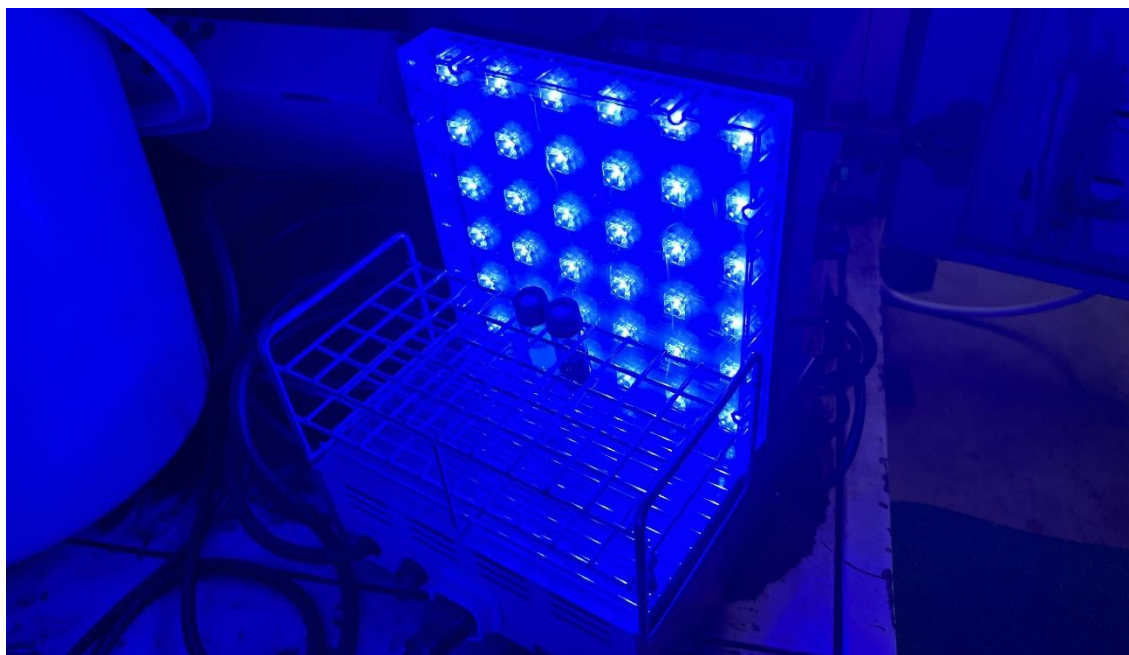
Figure S3. Standard LED setup for photochemical reactions (front view).
