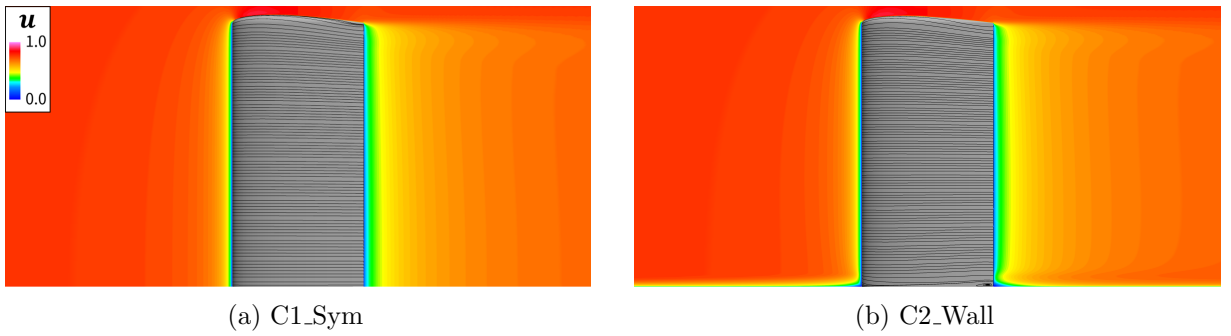
Figure 5.10: Streamwise velocity distributions on the x-y cross-section at z = 0 for M_\infty = 0.77 .
