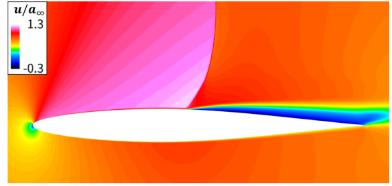
Figure 3.3: Streamwise velocity distribution at 4.0 deg for the stationary airfoil.
