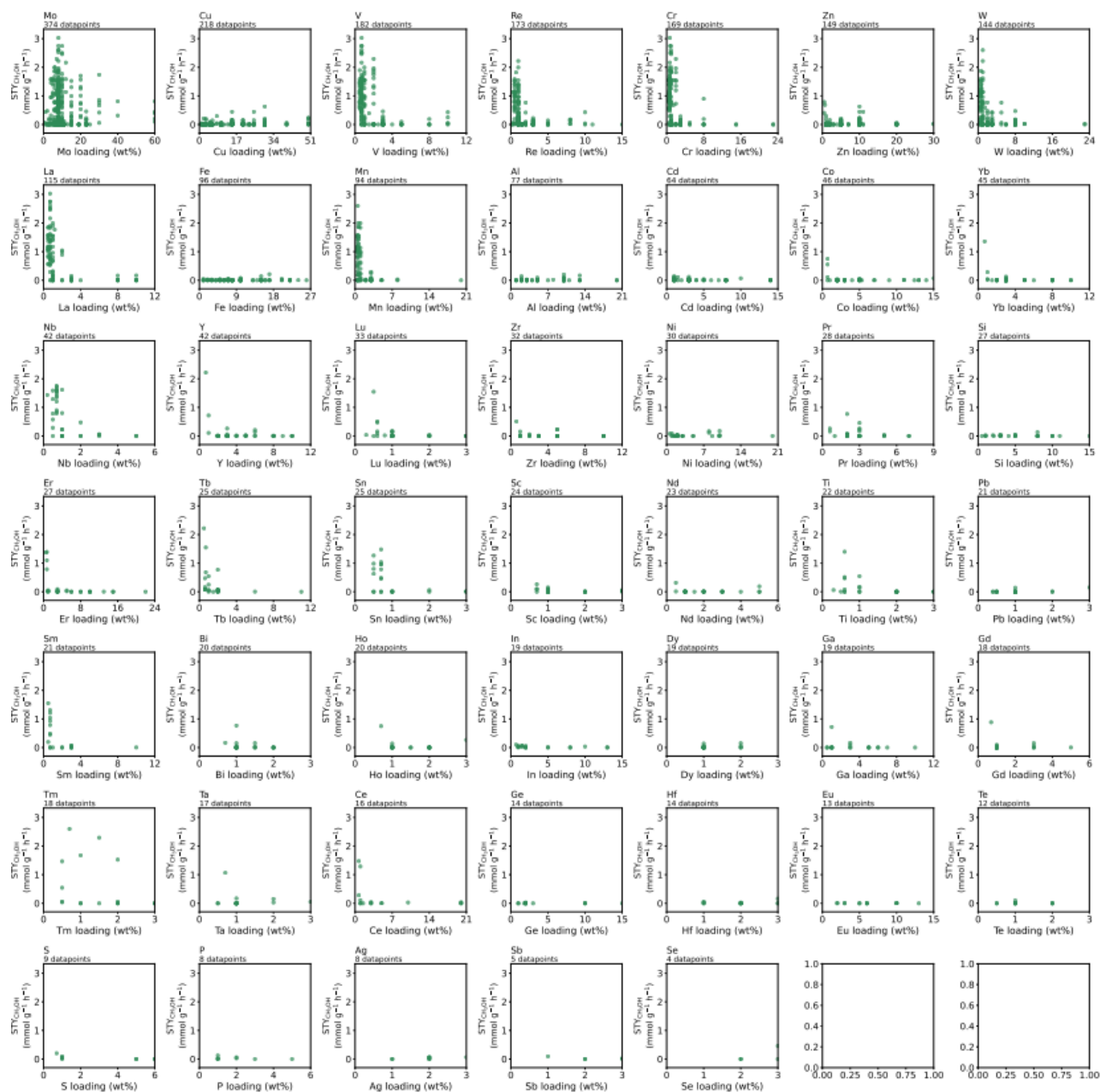
Figure 4.11. Effects of the loading amount of Additive elements on the \text{CH}_3\text{OH} formation rate.
