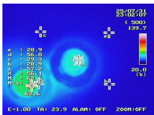
Figure S7. Thermographically derived temperature (62.6 ^{\circ} C) inside the milling jar after grinding for 60 min at 30 Hz.
