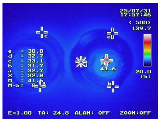
Figure S6. Thermographically derived temperature (41.6 ^{\circ} C) inside the milling jar after grinding for 60 min at 30 Hz.
