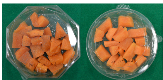
Fig. 2 Spoilage of fresh-cut melon cubes in polylactic acid (PLA) and polyethylene terephthalate (PET) containers at 10°C on the 10 th sampling day (right: PLA, left: PET)
