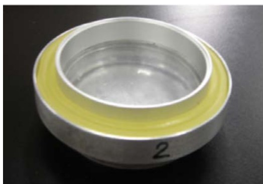
Fig. 2-15 Cup equipment based on Japanese Industrial Standard
