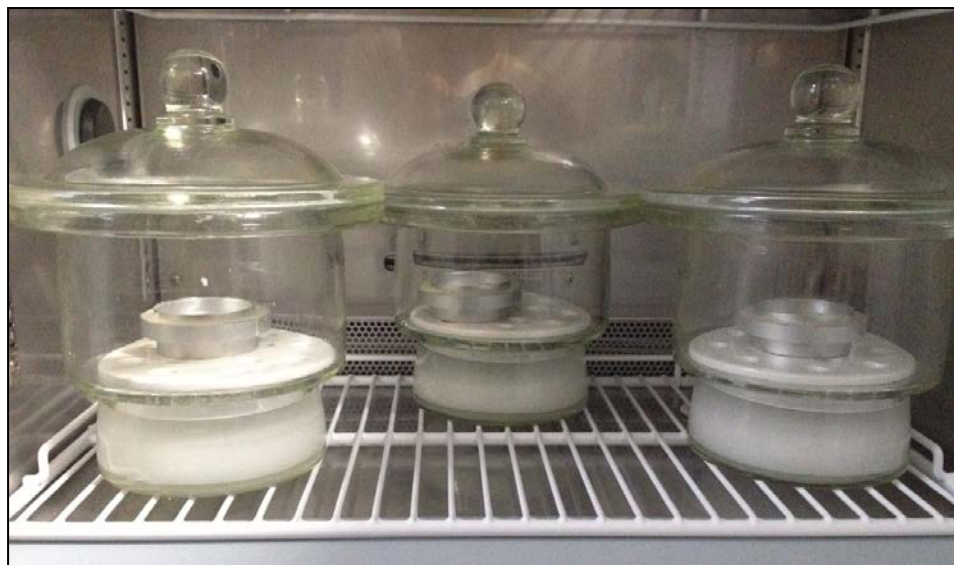
Fig. 2-17 Wet cup maintained in incubator
