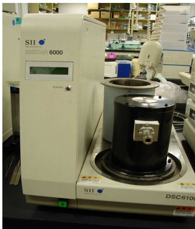
Fig. 2-2 Differential Scanning Calorimetry
